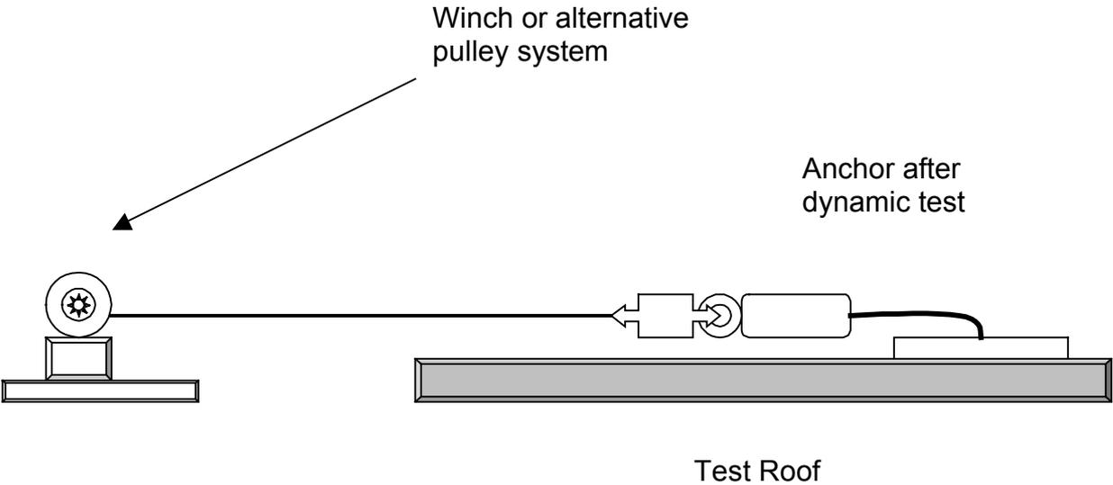
**FIG 3 – STATIC TEST ARRANGEMENT - TYPICAL**
