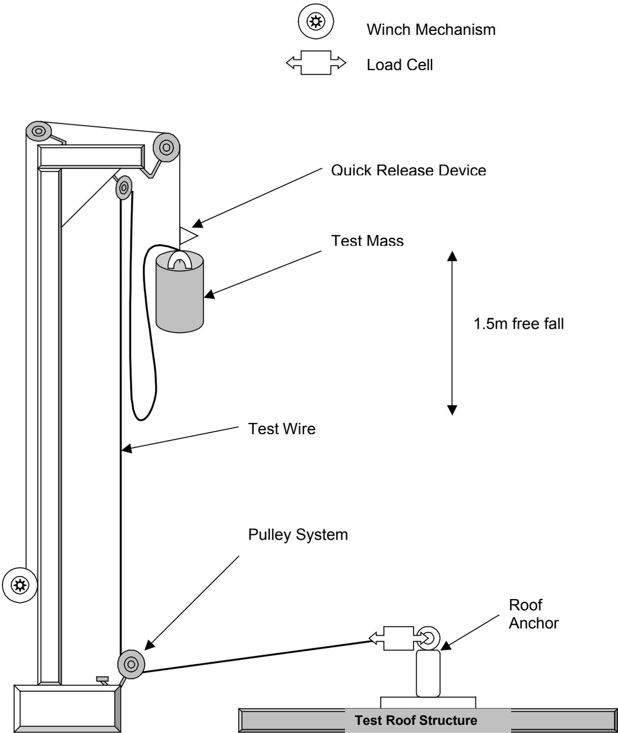
**FIG4 – TYPICAL DYNAMIC TEST SET UP**
