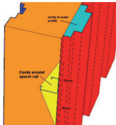
Fig 34: Unventilated cavity within the spacer rail and slightly ventilated cavity within the outer profiles
