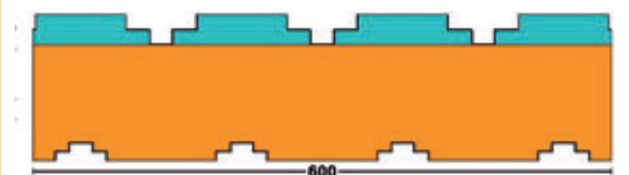
Fig 37: Cross section of model to calculate wall U-value
