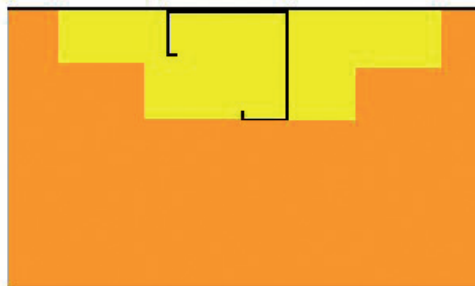
Fig 5: Approximation of the triangular cavity around a spacer rail by a series of steps
