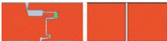
Fig 24: Detailed cross section of a composite panel joint and the simplified model to give the equivalent heat flow
