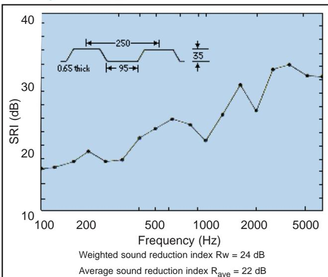
Fig 5 Sound reduction of a profiled metal sheet
