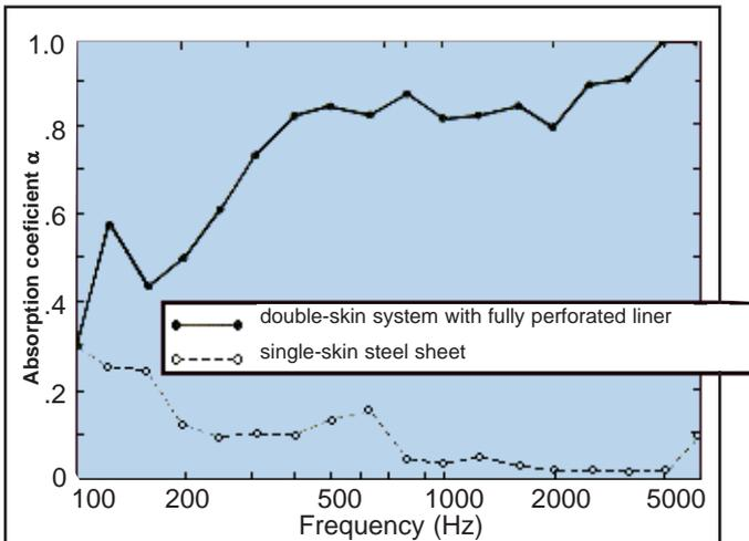
Fig. 14 Comparing sound absorption coefficients of a single skin cladding and a double skin system with perforated liner.
