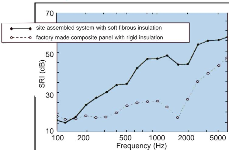
Fig. 12 Comparing a site assembled system and a composite panel.
