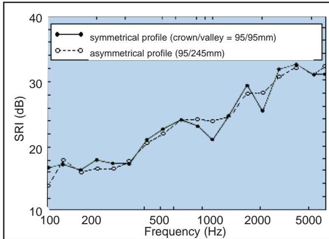
Fig. 6 Effect of profile shape or symmetry
