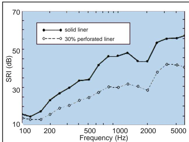
Fig. 15 Effect of perforated liner on sound insulation of a double skin system.
