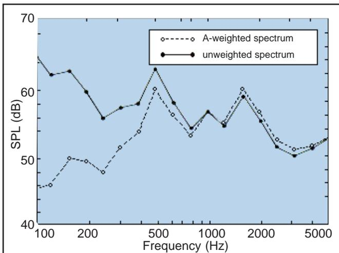
Fig. 3 Typical unweighted and A weighted noise spectra.
